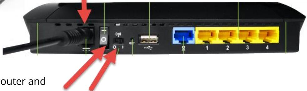
3. Turn ON the router and flip the switch to ( I )
