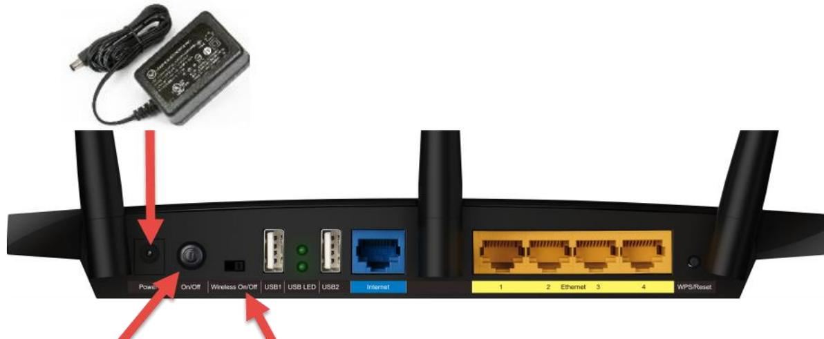
Push the button **IN** to turn ON the router.
